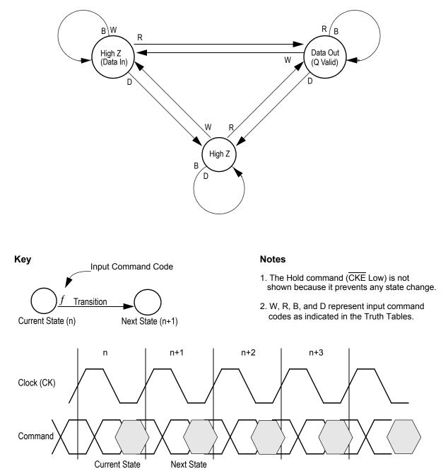
Current State and Next State Definition for: Pipelined and Flow Through Read Write Control State Diagram
